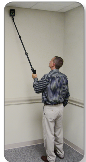
Telescoping antenna pole extended.
