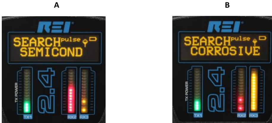
ORION 2.4 COMPARISON OF HARMONIC LEVELS
