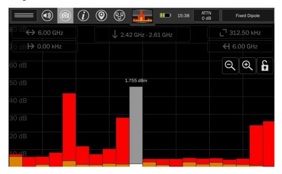
Tapping a selected SmartBar will zoom in to the portion of the spectrum represented by the span of the selected SmartBar. Again, the portion of the spectrum will be displayed as 20 sub-bars of equal power.
