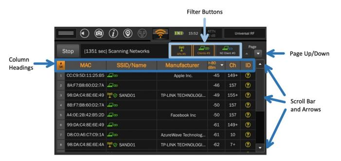
Any time after the initial 15 seconds, pressing the **STOP** button will pause/stop the scan. The user can then proceed to **Evaluating the WiFi Scan Results** (see next page). (Again, a longer scan time will allow the MESA to log more devices.)
