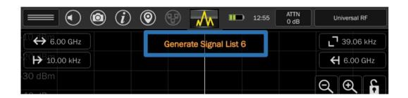
The MESA will analyze the peak reference trace, establishing an average baseline. Any frequency that crosses the set threshold level will be added to the signal list.
