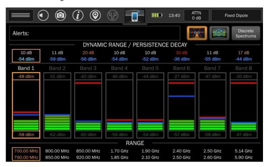
Each bar graph represents the power within a specified frequency band and there is an associated min, max, peak, and persistent power shown. Above the bars is an associated number for dynamic range (equal to  $P_{max} - P_{min}$ ) and persistent power (moving average). Above and below the bar graph shows the min and max powers. Within each bar graph, the blue and red bars indicate the persistent and peak powers respectively. The frequency range is displayed below the bar.
