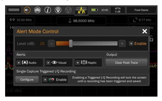
**Threshold Level** - Use the slider bar to set how far above the initial reference trace a signal should be before it triggers an alert. To begin receiving alerts check the enable box beside the threshold level adjustment. The threshold level must be adjusted before the enable box is checked.
