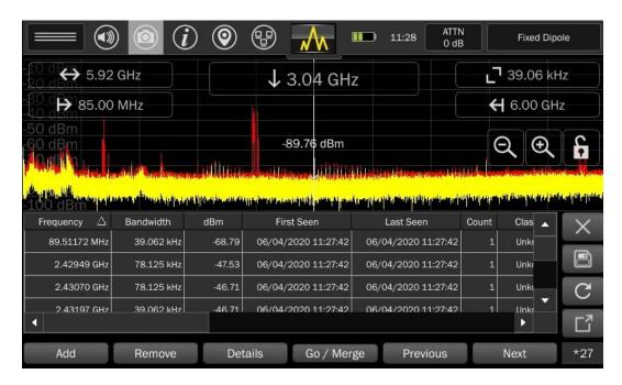
The signal list appears below the Spectrum window. The following sections provide details on signal list operations.
