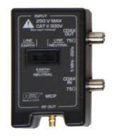
power conductors, a voltmeter should be used to measure the voltage across the conductors. If this voltage exceeds 250 volts, do not test with the Carrier Current Probe. Two power plugs are included for connection to US-style or Euro-style outlets. The included alligator clip cable assembly should only be used on 50V or less. Measurements can be made with three different pair configurations using the switch on the front of the carrier current probe: Hot/Neutral, Neutral/Ground, and Hot/Ground.
