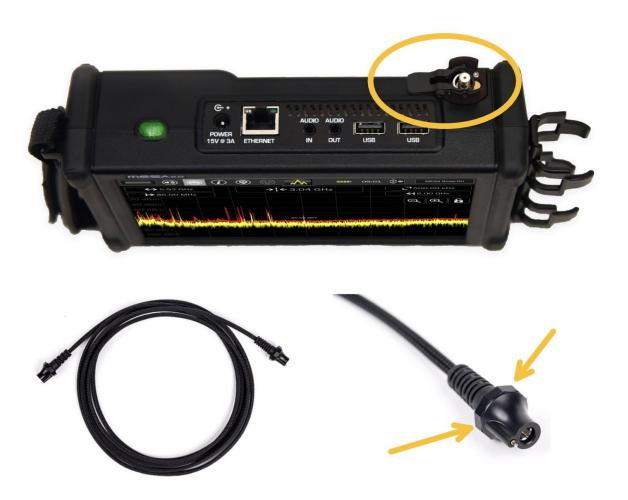
Note: When disconnecting the powered connector cable, **pull from the cable release for leverage**. *Do not pull from the cable*. Doing so could damage or shorten the life of the cable. It is not necessary to power off the MESA 2.0 when changing probes/antennas. The MESA 2.0 provides a quick-release mechanism to help with removing cables. Press down on the quick-release lever while simultaneously pulling from the cable release for leverage.
