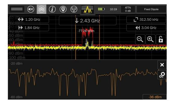
The RSSI option in the Mode Settings Menu turns the RSSI feature on. The spectrum portion of the graph will be compressed and displayed on the top half of the screen. The RSSI feature will be displayed on the bottom half of the screen.
