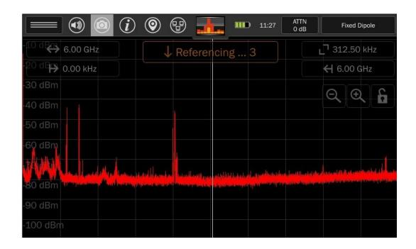
Note: During the collection of the reference trace, the screen can be locked with a pin code to prevent tampering with the collection of the reference trace. Press and hold the lock icon on screen for at least 5 seconds. Then follow the onscreen prompts. For additional details regarding locked monitor mode, see page 90.
