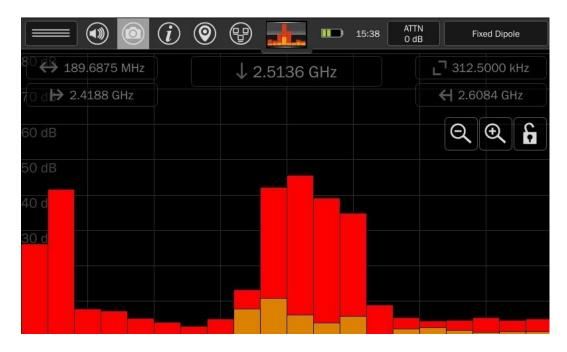
Notice the spectrum indicators at the top of the screen (span, start frequency, stop frequency). These will change to indicate the new span.
