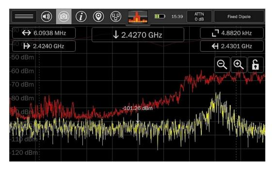
(To return to the SmartBars view, repeatedly press Zoom Out until the displayed span is greater than 200 MHz. Changing the Span directly by tapping the Span Indicator at the top of the screen and changing the value to one that is greater than 200 MHz will also accomplish this.)
