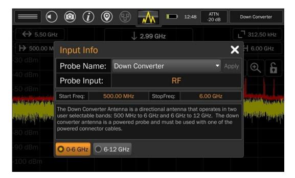
In the lower bottom of the Input Info dialog, the  $\mathbf{0} - \mathbf{6}$  GHz and  $\mathbf{6} - \mathbf{12}$  GHz buttons select between bands. The start and stop frequencies change depending on the down converter state. After selecting the desired band, press the "x" to close the Input Info dialog box.
