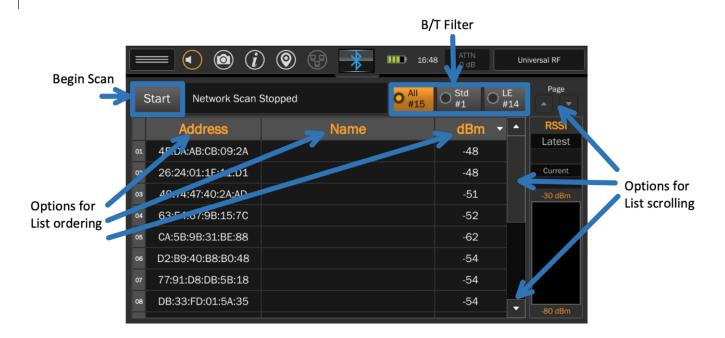
Scroll through the list by tapping the up/down arrows or tap-and-hold on the bar between them and drag it up or down. There is also a page up/down button located on the top right of the display below the status bar. Individual devices can be highlighted. In addition, devices can be filtered into **All**, **Std.**, and **LE** by selecting each button. This can be done both during the scan and after the scan is completed.
