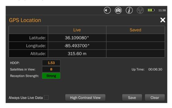
Note: In order to receive GPS coordinates, the GPS Adapter (see page 18) must be inserted into one of the MESA's USB ports. To improve GPS reception, especially on cloudy or overcast days, use a USB extender cable to physically locate the GPS adapter further from the MESA unit.
