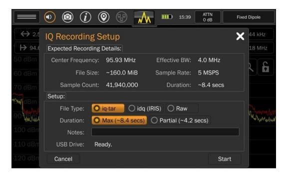
Note: The I/Q Recording option is only available in the Mode Settings Menu at spans of 14 MHz and below. The circle around the sound icon will be gold when it is available. A trigger-based I/Q Recording is also available on the MESA 2.0 (see page 35).
