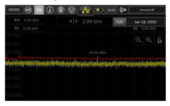
Tapping the time display in the status bar will open a small dialog box with the date. Press "Edit" in this dialog box to set the time zone, time, & date for the MESA.
