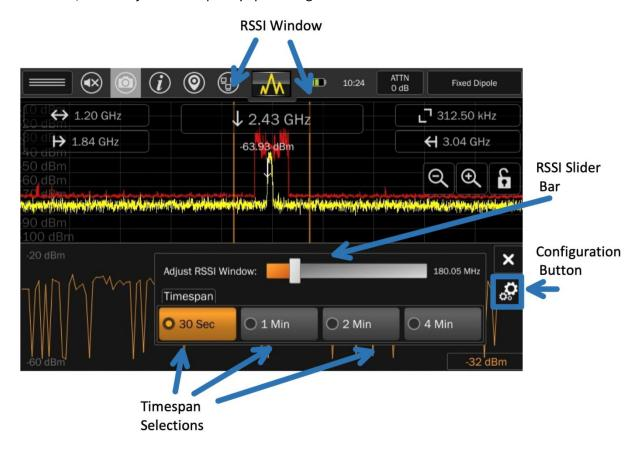
The RSSI Window can be adjusted by tapping/selecting the *Configuration* button in the RSSI graph. Use the slider bar to adjust the window.
