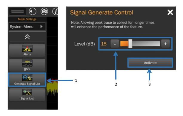
The reference peak trace will collect for a minimum of five seconds. After this, continue collecting the peak trace for as long as desired. The longer the peak trace is collected, the more accurate it will be and the more likely it will include any suspect signals present.
