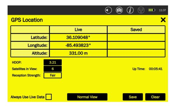
GPS coordinates are not very well received indoors. For this reason, the GPS location feature enables the user to use saved GPS coordinates for tagging saved data and signals. To use Saved GPS Coordinates:
