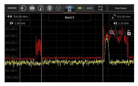
Tap any of the discrete bands to select it. The selected band will be highlighted with an orange border. The spectrum indicators at the top of the screen (span, start frequency, stop frequency) will change to reflect the correct values for the selected band. The name of the selected band will be displayed at the top center of the screen.
