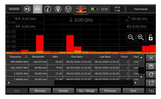
A merging algorithm is employed so that over time signals such as frequency hoppers or FM transmitters, which initially appear as several distinct, closely spaced signals are eventually grouped into one signal with a larger bandwidth as the envelope of this signal begins to fill in with peaks. Generation of this signal list continues, adding any newly detected signals to the list until Spectrum Mode is achieved via zooming in or until SmartBars Signal Resolution mode is exited.
