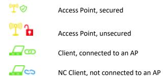
If AP/Client device names are available, they will be listed beside the symbol. However, a name in blue indicates an NC Client's probe request and *not* the actual device's name. An NC Client is not connected to an Access Point. (For more on how the MESA 2.0 classifies devices, see page 72, #3).
