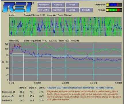
In conclusion, the ASA software provides a useful method for setting up, testing, and calibrating a noise masking system. Furthermore, it should be noted that the concept of White Noise, Pink Noise, and blanket noise masking become very vague when considering several important facts:
