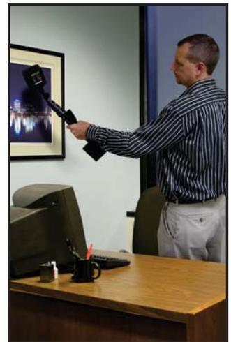
Transmit power and both 2<sup>nd</sup> and 3<sup>rd</sup> harmonic LED level indicators are located on the antenna head for line of site display so the user can see response activity in line with the target area being swept. System and operational status (TX Power mode, Frequency mode, Audio options, etc.) is also displayed on the antenna head and controlled via the keypad on the handle.
